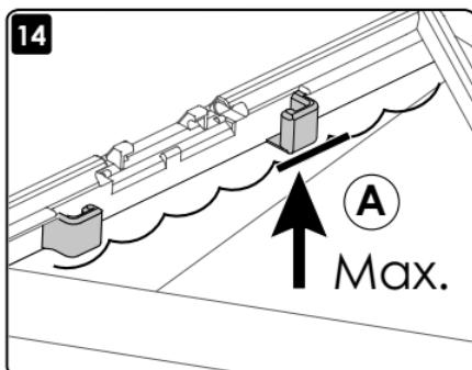
UK • Make the "drip curve" so that the water does not come into contact with the socket.
